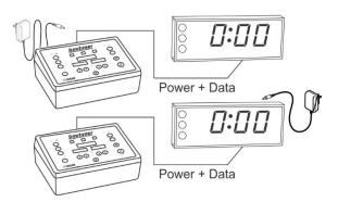
For cable runs greater than 1000-feet, always provide local power to the signal light using the included 1-Amp power supply (center pin +).
