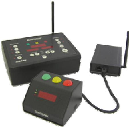
Note: Limitimer PRO-200RF cannot be used in proximity to DSAN cue lights because both products transmit on the same radio frequency.
